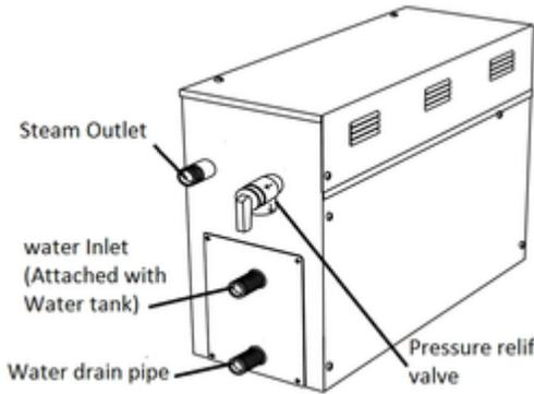
The steam generator should not be installed in the steam room. Install in a dry place where the ventilation is good.
