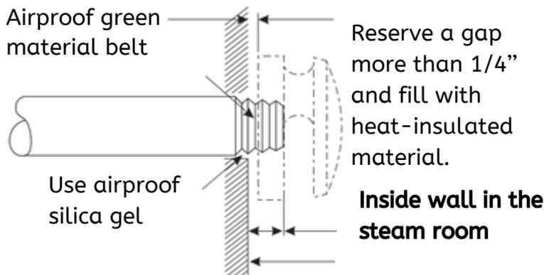
The pipes, its accessories and the holes should be air proof by applying glue so that no steam will enter the holes in the wall.
